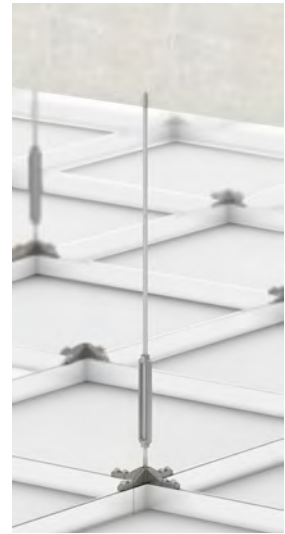
Tate Grid hanging method from concrete building
