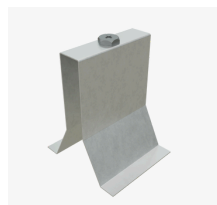
Security Hold Down Clip Hold down clip that prevents removal of tiles below the ceiling for security. Hold down clips should be used on all edges where the tile has been cut. Clip can be cut on-site to suit perimeter installation.
