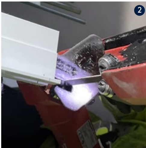
Figure 10.. Field coping with a band saw. Images 2 & 3
