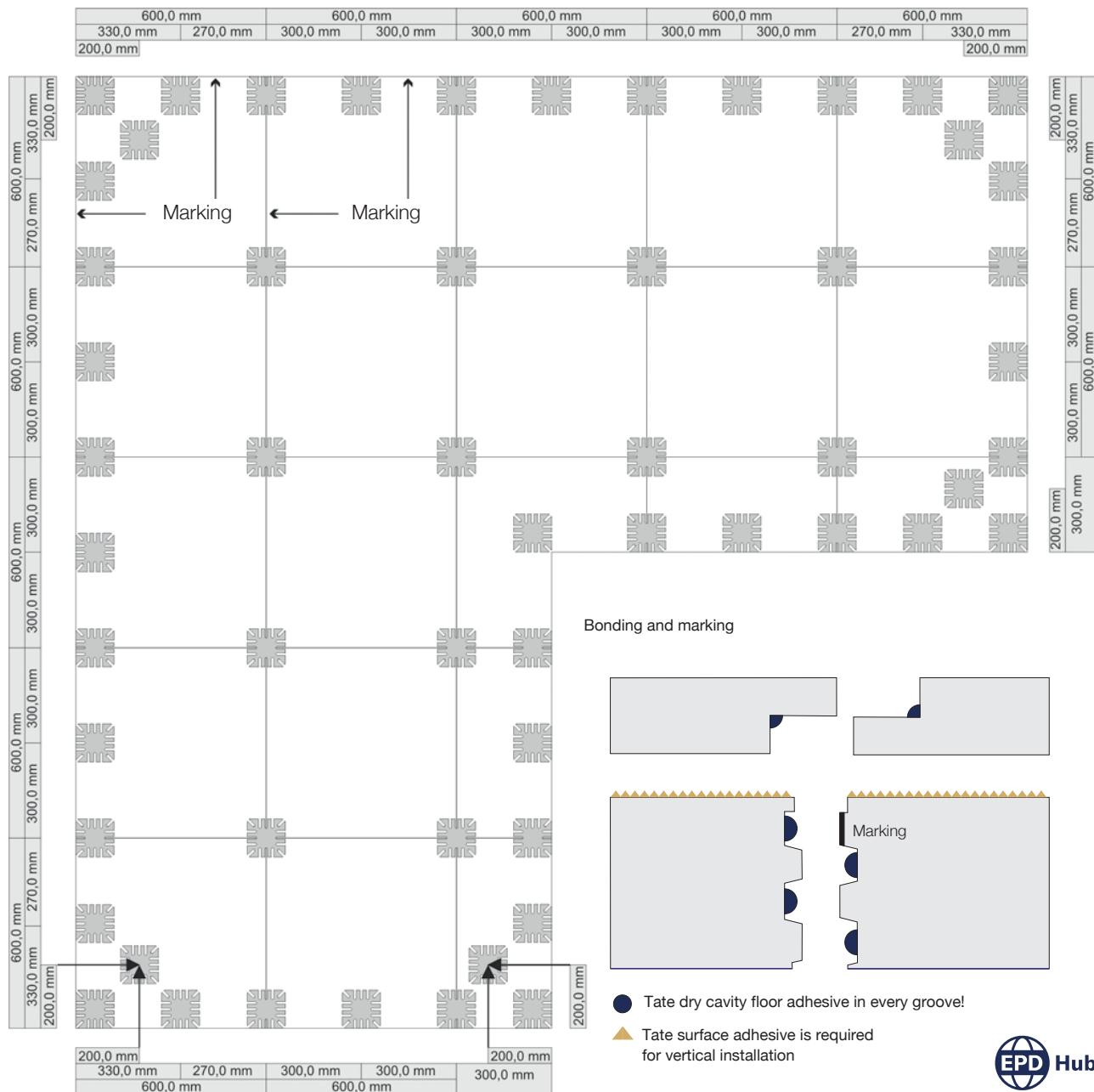
Pedestal layout: Care must be taken to ensure that the corner pedestals are positioned at a distance of 200 mm from the centre of the pedestal head to both edge joints. This positioning must be strictly observed.
