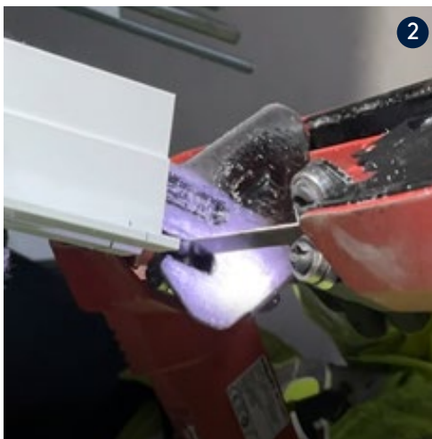
Figure 10.. Field coping with a band saw. Images 2 & 3
